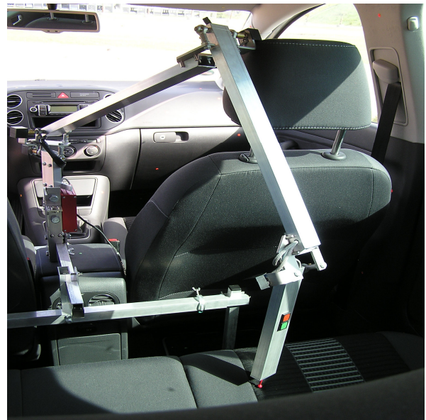
Fig. 3: The digitizer to capture the 3D coordinates of the vehicle interior and the location of the measurement points.
