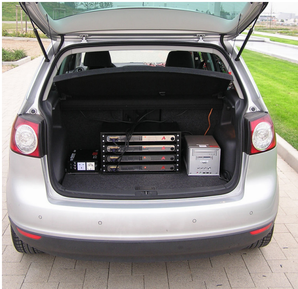
Fig. 5: 96 channel data acquisition and recording equipment inside the trunk.
