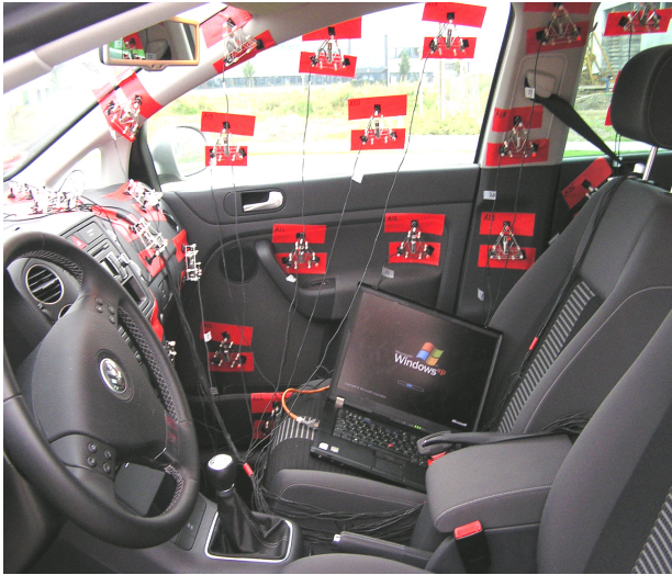
Fig. 4: The PU probes are spatially distributed.
