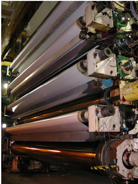
Figure 3. Supercalender Section Being Studied
