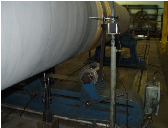
Figure 19. Orthogonally Setup LVDTs Against Roll Surface
