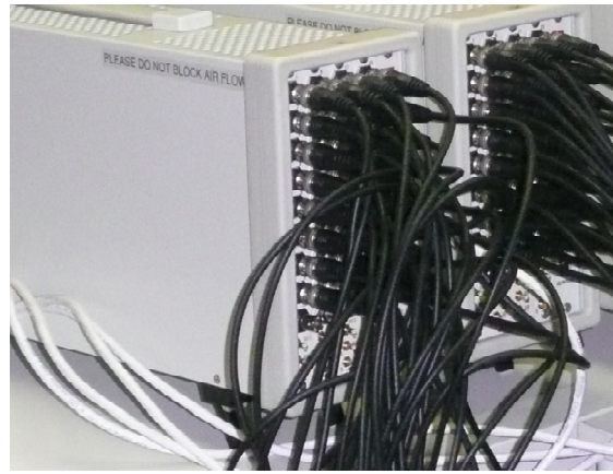
Figure 5. Multiple DSPCentric Abacus Chassis Networked for Larger Channel Count Field Data Acquisition and Analysis
