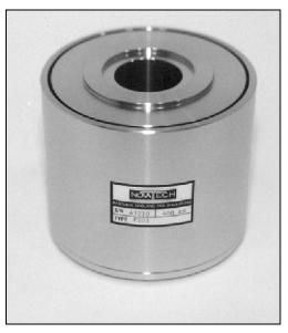
Geometry: Axial strain cylinder in weather sealed case, with raised end load bearing faces and hole right through. For use in compression or in fail-safe tensile applications.
