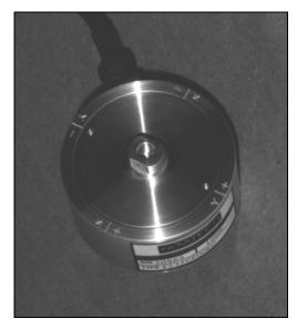
The F232 measures forces in two axes at 90° and the F233 measures forces in 3 mutually perpendicular axes. Apart from error evaluations, each output is pure and requires no mathematical manipulation. The loadcell is moment sensitive requiring calibration to be carried out at a specified force centre. The standard centre is specified in the specification. If this is not suitable for your application please consult our engineering department about alternative calibrations.
