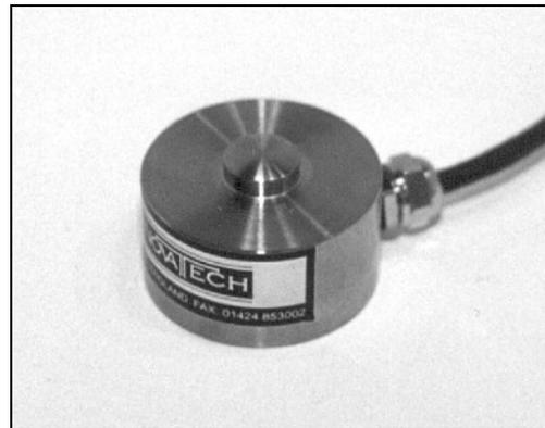
The F303 is aimed at the volume OEM user who requires a reliable high quality axial sensor at a low price for low accuracy compressive force measurement in equipment. It is manufactured from stainless steel and sealed to IP65 for long life in typical industrial operating conditions. The sensor is designed for simple mounting on a smooth flat surface.
