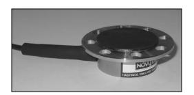
The F304 is a compact, high accuracy low profile loadcell for measuring brake pedal application forces. The loadcell is robust in construction with a maximum force range of 2500N (250kg). Its multi-hole fixing allows simple attachment to any shape pedal using screws or cable ties. The low profile stainless steel design maintains the brake pedals ergonomic geometry.
