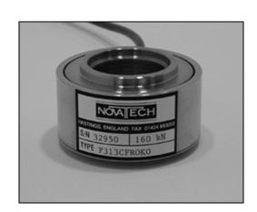
Geometry: Axial strain cylinder in weather sealed case, with raised end load bearing faces and hole right through. For use in compression or in fail-safe tensile applications on a wide range of OEM or end-user applications.
