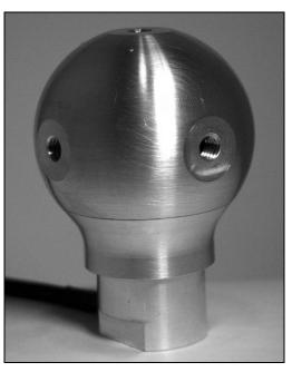
The F321 gear shift loadcell measures gear lever forces required to achieve gear selection. An ergonomically designed gear knob senses the force from a human hand or a mechanical actuator. The three axis force components are represented by three pure loadcell output signals. The gear shift loadcell is supplied calibrated and ready to use, no in-situ calibration or mathematical computation is required.
