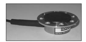
The F322 is a compact, high accuracy low profile loadcell for measuring accelerator pedal application forces. The loadcell is robust in construction with a maximum force range of 250N (25kg). Its multi-hole fixing allows simple attachment to any shape pedal using screws or cable ties. The low profile design maintains the accelerator pedals ergonomic geometry. Low mass aluminium alloy construction reduces the mass influence upon the accelerator pedal in dynamic testing.
