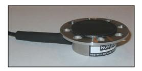
The F323 is a compact, high accuracy low profile loadcell for measuring clutch pedal application forces. The loadcell is robust in construction with a maximum force range of 1kN (100kg). Its multi-hole fixing allows simple attachment to any shape pedal using screws or cable ties. The low profile design maintains the clutch pedals ergonomic geometry. Low mass aluminium alloy construction reduces the mass influence upon the clutch pedal in dynamic testing.
