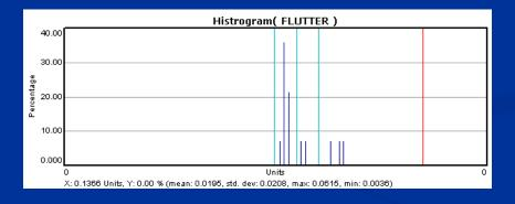
The envelope value H2 is a measure of the "flutter" defect. The ratio for the good parts to the "flutter" parts was more than 11 to 1.
