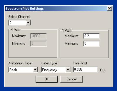
Allows annotation of spectral peaks by amplitude or frequency
