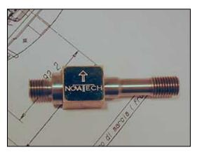
Novatech Measurements proactively proposed a loadcell system to measure braking torque when applying the brakes of a Formula 1 racing car. Typically, a 3kNm braking torque produces a 20kN reaction at the brake calliper; this was shared between two 10kN loadcells. High temperatures in this application required a loadcell with a safe working temperature of between -10 and 250°C. The loadcell system would also be subjected to high energy vibrational and shock loads at high temperatures.
