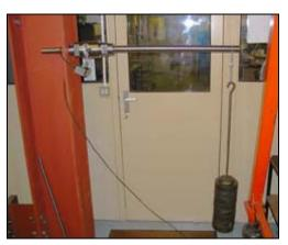
The customer required a number of loadcells for fatigue testing of airframe structures. The loadcells themselves would be subject to the same cyclic loads as the structure under investigation and therefore must be built to withstand these tests.
