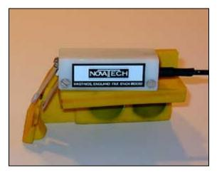
A system was required by the customer to measure panel gaps of a road car tailgate. Normally a fixed wedge was used to set the gap but this did not take into consideration the nature of the closing force required.
