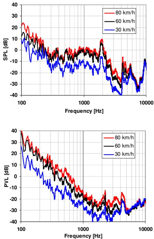
**Figure 6:** Autospectrum of the external noise only (speaker turned off) relative to the autospectrum at still standing conditions (speaker on). Top: pressure, bottom particle velocity response.
