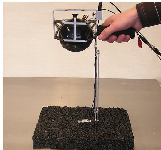
**Figure 1:** Handheld PU in situ impedance setup in the laboratory
