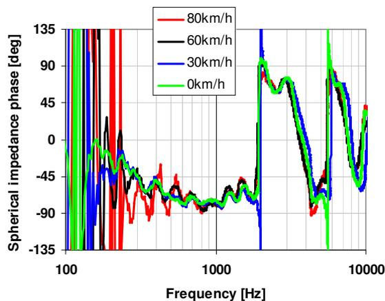
Figure 5: Measured impedance phase at different speeds
