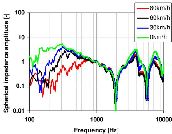
Figure 4: Measured impedance amplitude at different speeds
