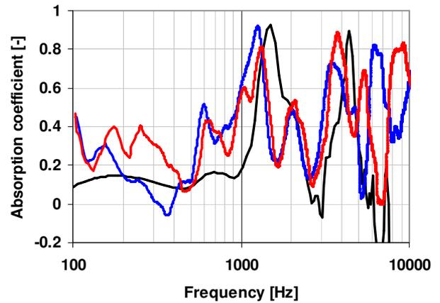
Figure 2: Examples of PU absorption measurements on asphalt
