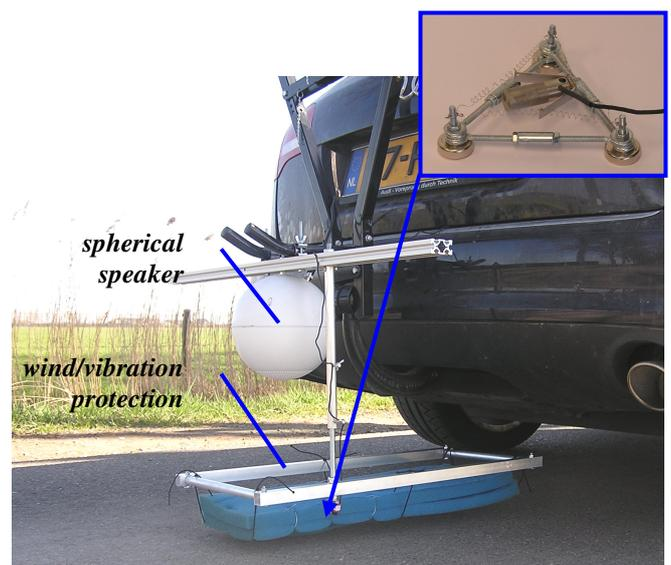
Figure 3: PU surface impedance setup mounted behind a car
