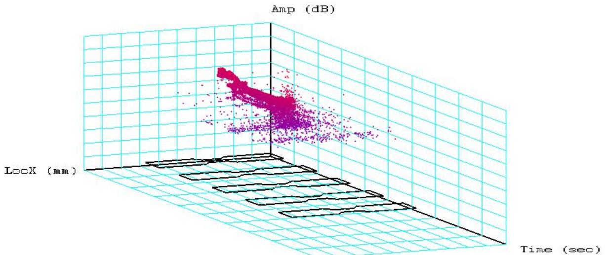
Figure 15 3D representation of AE events showing their distribution in time and space in TRIP steel
