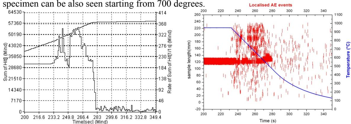
Figure 10. AE events (rate and localization in Cr-Mo steel at the beginning of cooling
