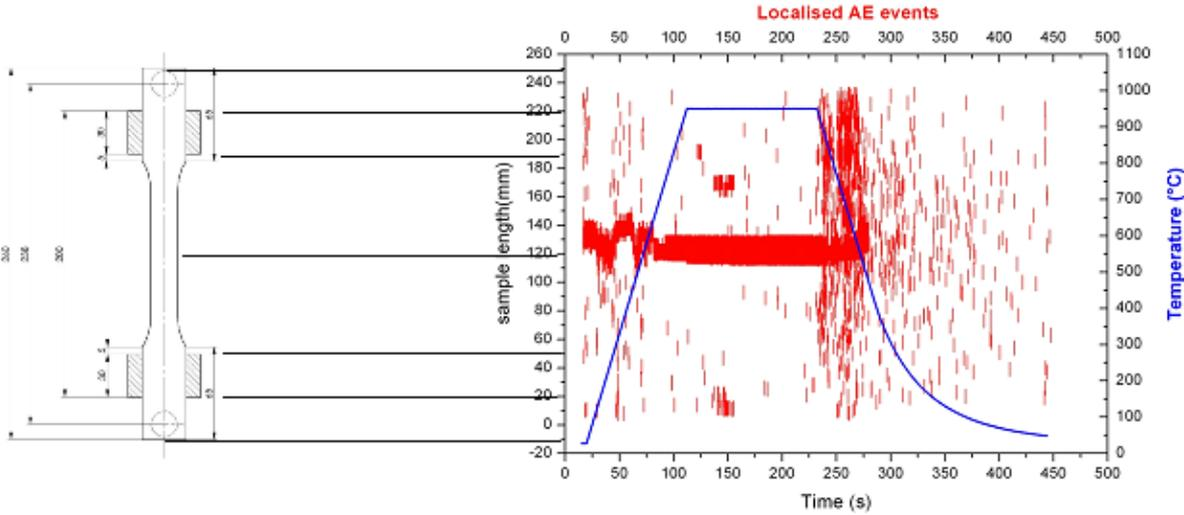
Figure 8. Localization of AE events on a Cr-Mo steel during heating up and cooling down
