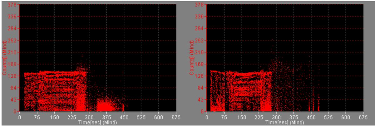
Figures 13 and 14. Counts (characterising number of oscillation within the AE event) for TRIP and Cr-Mo steels correspondingly
