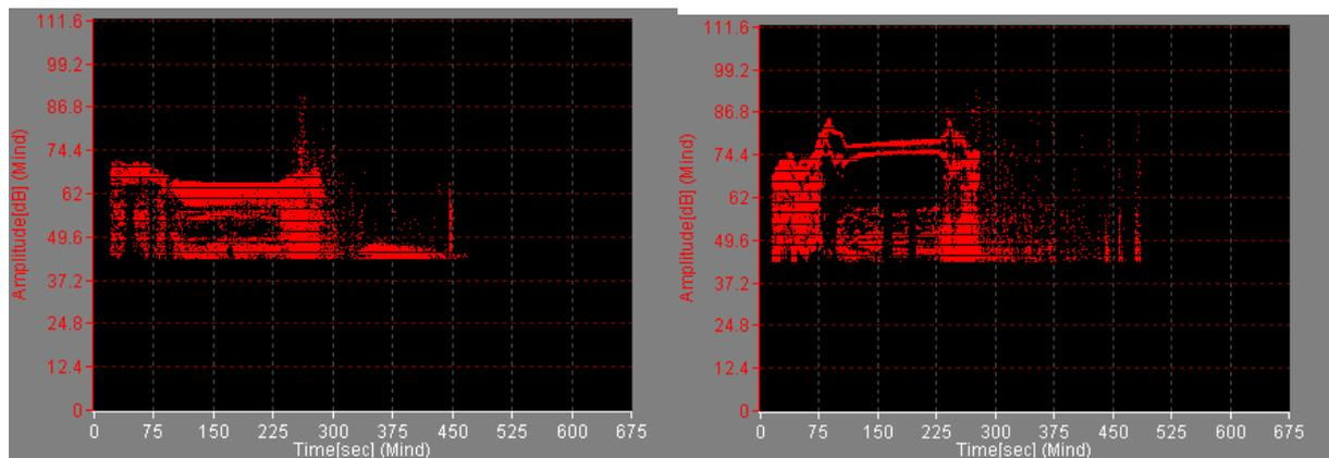
Fig 11 and 12 Changes of amplitudes of AE events during heating up and cooling down in TRIP and in Cr-Mo steels
