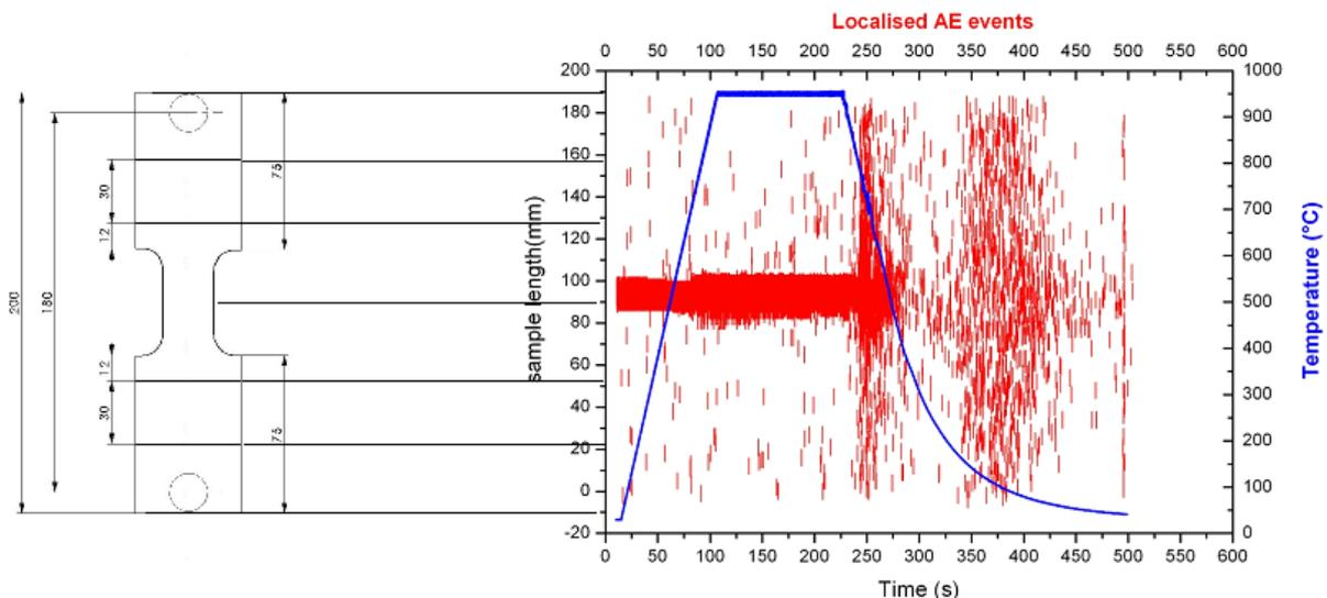
Figure 7. Localization of AE events along the specimen during heating and cooling in TRIP steel
