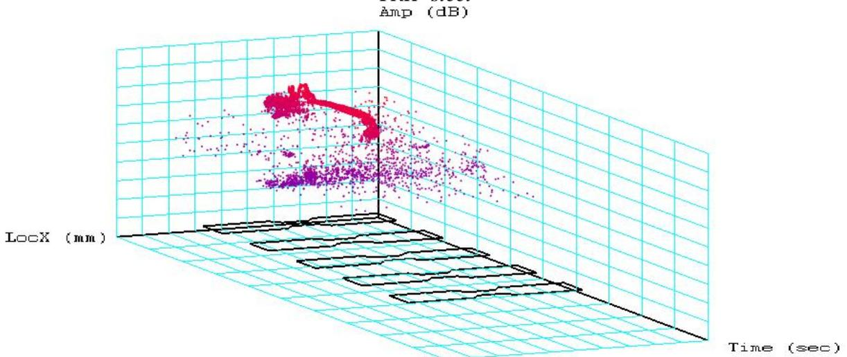
Figure 16 3D representation of AE events showing their distribution in time and space in Cr-Mo steel
