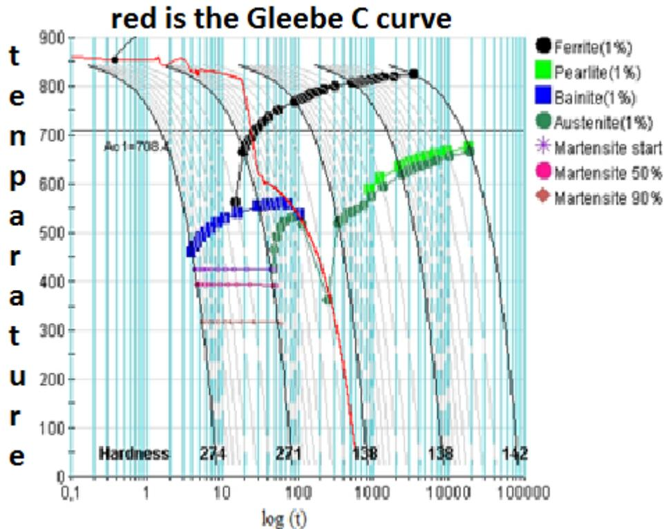
Fig 17. Calculated phase transition curves for fast cooling in Gleeble simulator (from [9])
