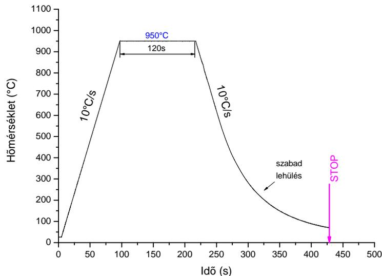
Figure 5. The temperature changes in single heating-cooling experiment
