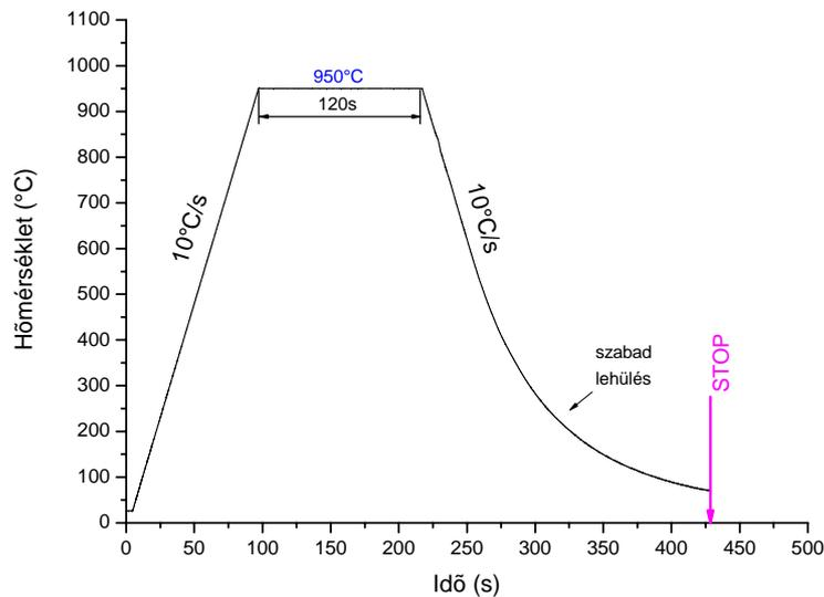
Figure 5. The temperature changes in single heating-cooling experiment
