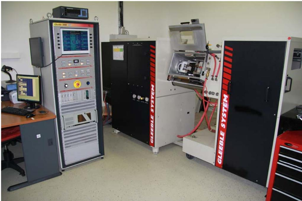
*Figure 1. Gleeble 3800 thermomechanical simulator*
