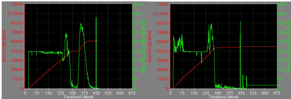
Figure 6. Comparison of rate of hits (green) and sum of hits (red curves) for TRIP and Cr-Mo steels during heating and cooling process
