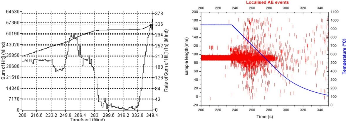
Figure 9 AE events and their localization at the beginning of the cooling in TRIP steel
