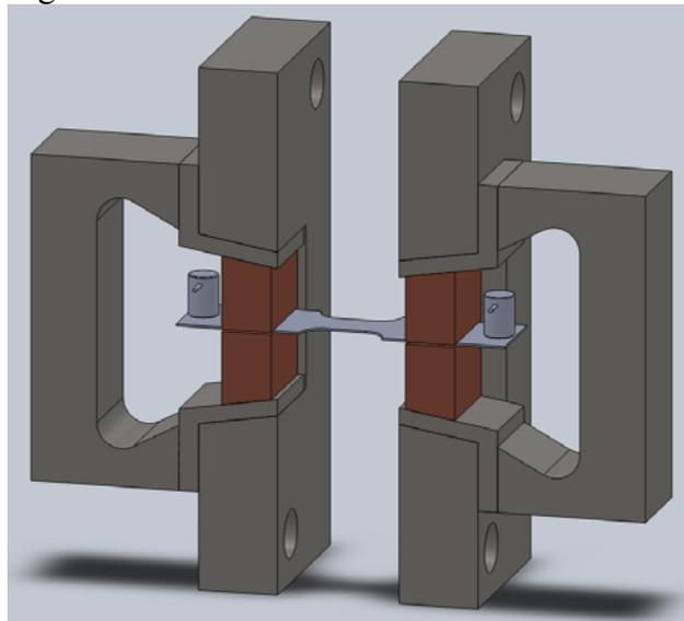
Figure 4. Specimen in the cooled jaws of Gleeble with two AE sensors
