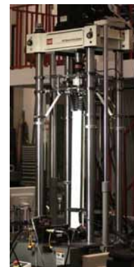
Setup for experiments on the composite beams. The beam is clamped at the top, the load is applied at the lower tip
