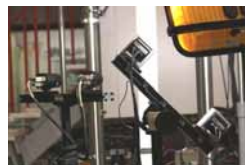
Setup of two DIC systems: Left – for warping measurements, right – for global response measurements
