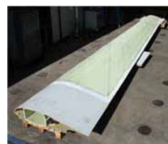
Modified blade section with extra UD layers
