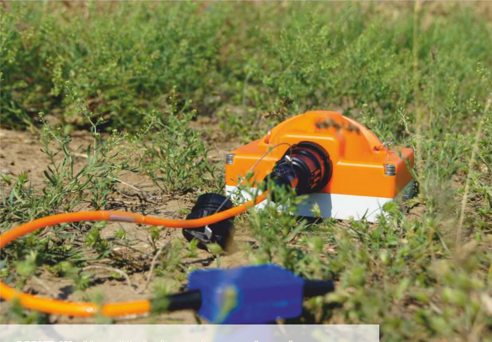
SCOUT. Working with single geophones and geophone group.
