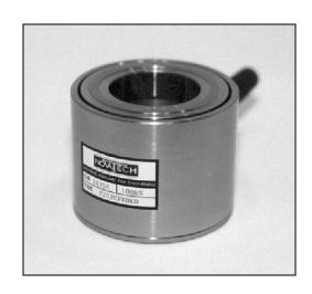
Geometry: Axial strain cylinder in weather sealed case, with raised end load bearing faces and hole right through. For use in compression or in fail-safe tensile applications.
