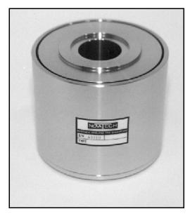
Geometry: Axial strain cylinder in a sealed case, with raised end load bearing faces and hole right through. For use in compression or in fail-safe tensile applications.
