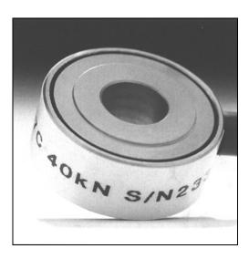
Geometry: Axial strain cylinder in weather sealed case, with raised end load bearing faces and hole right through. For use in compression or in fail-safe tensile applications on a wide range of OEM or end-user applications.
