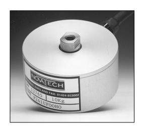
Geometry: Flexure strain assembly in cylindrical housing, open or weather sealed with end internal fixing. For universal use in tension and compression, with high compensation for off axis load inputs.
