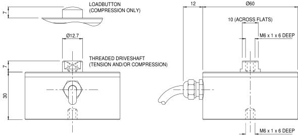
NB: The case height increases to 42mm on the overload stop version.
