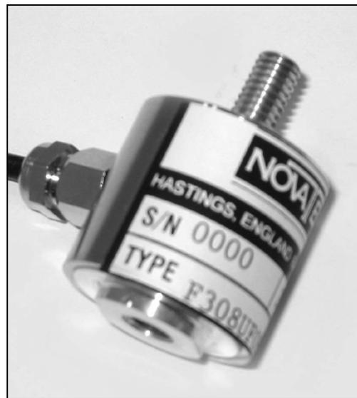
The F308 is a compact axial loadcell with improved EFI compared to diaphragm loadcells. The inert base and top fixings with spanner flats allow ease of installation. The strain geometry possesses a plane with good EFI performance defined as perpendicular to the loading axis and the spanner flats. This is particularly useful when a loadcell is used to support mass with its weight acting perpendicular to the measurement axis.
