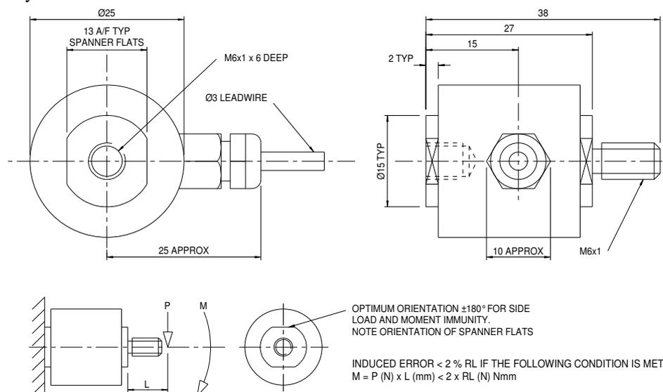
To optimise the performance the F308 end faces should be maintained parallel under load.
