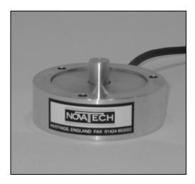
Geometry: Slender disc, with outer ring earth fixing and live inner boss usually shaft driven.
