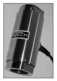
The F317 is a high performance cylindrical loadcell offering a high degree of output symmetry in compression and tension. A high slenderness ratio strain section improves all round performance compared to the older design F204. New thread sizes are employed offering more economic sizing of rod end bearings and improved availability. Novatech can supply suitable rod ends.
