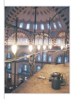
Sentez Electronic & Engineering Ltd were commissioned to set up a strong-motion experiment in the mosque, to record the response of the structure to ground movements and identify areas which will be susceptible to damage.
