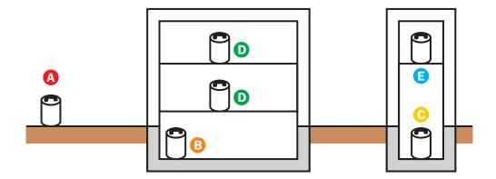
**Free field:** Location A measures the reference ground motion at a location distant enough that the effects of the structures are insignificant, but where the ground motion is still representative of that at the site.
