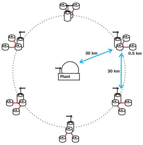
In this case, each station consists of one velocity sensor and three accelerometers. When two of any set of three accelerometers exceed their triggering threshold, the alert is given. Under normal conditions, continuous seismic data is recorded for basic research and monitoring purposes.
