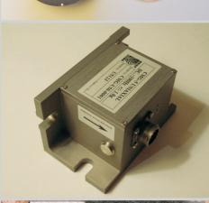
The 5TD offers support for high sample rates and low latency data transmission, as well as direct data download over FireWire. At-a-glance status information is available on its optional LCD display as well as being transmitted with the data streams in GCF format. Full configuration and firmware updates can be carried out remotely over the standard serial interface.
