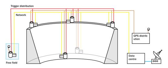
A digital sensor (such as the Güralp CMG-5TD) can perform **STA/LTA or level triggering** calculations, and output high rate streams when an event occurs. Using a dedicated **external trigger** network, the entire array can be triggered from any of the component sensors, ensuring that full data records are always available.
