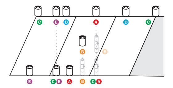
**Dynamic response:** Positions A; B for more detailed results. Instruments within the dam can be placed in boreholes (for earth dams) or galleries. **Tridimensional response:** Positions D, instruments placed at ½ points. **Effective input motion:** Positions C, instruments placed at the base of monoliths and at each side of the canyon.
