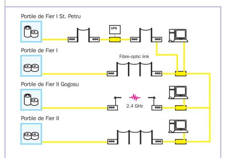
A further installation at St. Petru, near Portile de Fier I, contains a CMG-5T instrument and a CMG-40T-1 medium motion velocity sensor, with a DM24 and DCM configured similarly to the dam installations.
