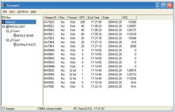
Using Scream!, operators can also **configure and control** Güralp digitizers remotely.
