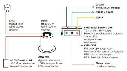
Stations using any of these options can be combined to form the full array. Where arrays are installed during dam construction, a **local area network** is often installed as part of the basic infrastructure. Alternatively, **RS232**, **RS422**, **fibre-optic**, **Wi-Fi** (**802.11b**) **or radio links** can be used. Wireless technology is particularly attractive where laying dedicated cabling would be impractical, or for temporary experiments.
