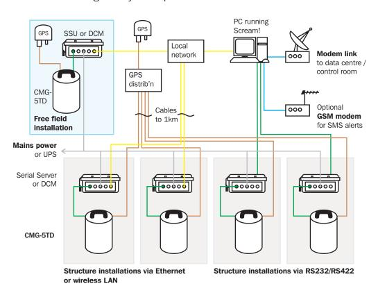
A PC running Güralp Systems' **Scream! software** can collect data from any number of sources and archive it to a local hard disk, or retransmit to a data centre further afield. Scream! can **convert data** into a number of common formats, including MiniSEED and UFF.
