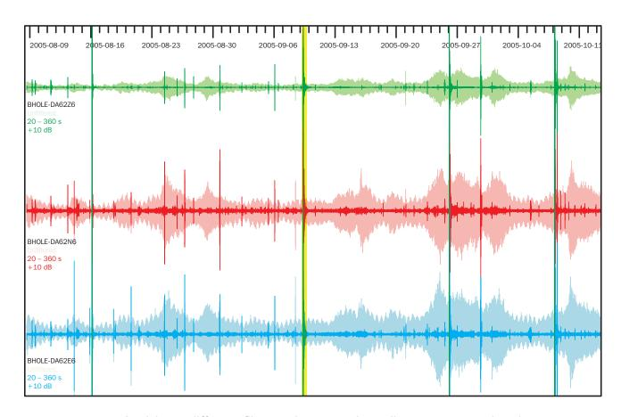
Applying a different filter to the same data allows us to examine the teleseismic events recorded during this period. In the graph above, a  $20-360\,\mathrm{s}$  filter has been used. Again, the raw data is included for comparison.
