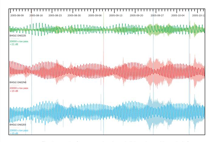
The data on the front page, also shown in lighter tint on this graph, is from a CMG-3TB 360 s - 100 Hz sensor installed in our test vault in Wolverton, UK. 10 weeks of continuous data streams were recorded at a rate of 1 sample/s.
