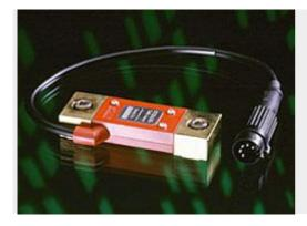
The bolt-on is machined from high-performance tooling steel which is thermally compatible to most cast and structural steels in respect of temperature coefficients. The machined sensors are heat treated to give you, the customer, optimum performance and stability. The SPL4000 sensors are cycled through a wide variation of temperature changes and are compensated against and thermally induced errors.
