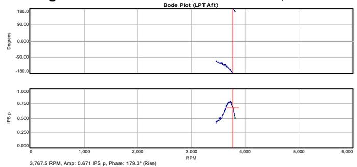
Figure 5. Bode Plot of LPT Vibration Data, Run 1
