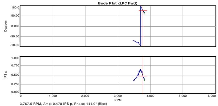
Figure 4. Bode Plot of LPC Vibration Data, Run 1
