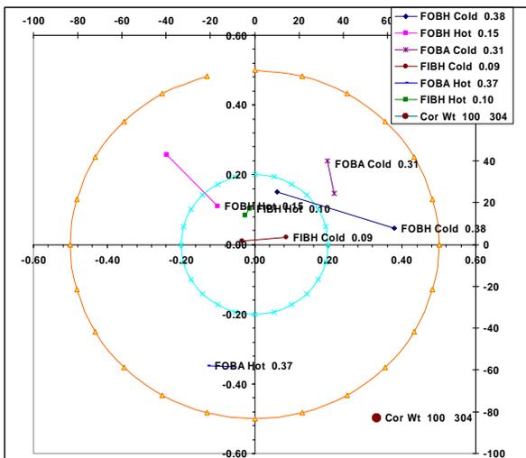
Figure 10. Fan 105 Recommended Balance Corrections and Resultant Vibration Vectors
