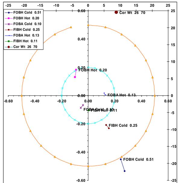
**Figure 8. Fan 108 Predicted Trim Balance from Last Good Correction (145 gm @ 270 degrees)**
