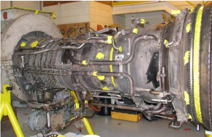
Figure 1. GE LM5000 Gas Turbine on Stand
