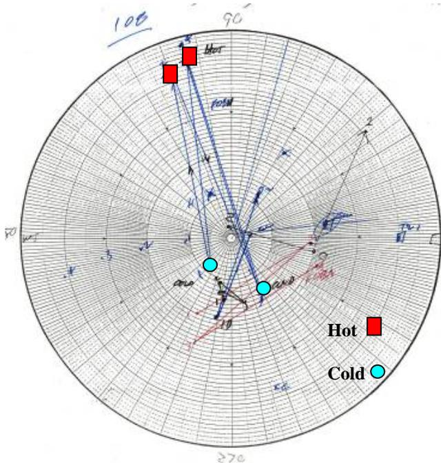
**Figure 7. Fan Vibration Changes with Thermal Excursions Demonstrate Repeatability**
