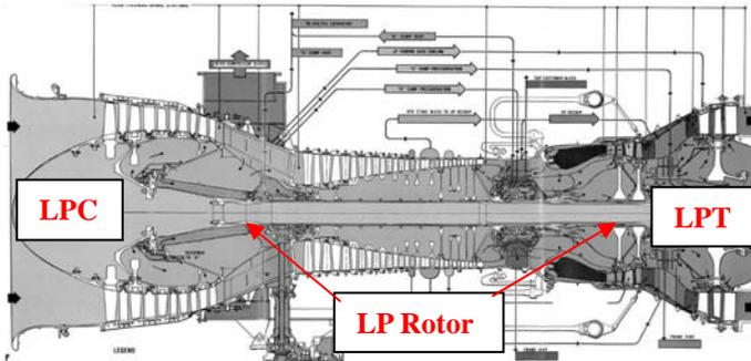
Figure 2. Schematic of GE LM5000 Gas Turbine (from GEAE)
