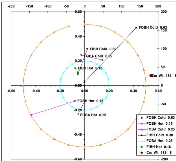
Figure 9. Fan 107 Recommended Balance Corrections and Resultant Vibration Vectors
