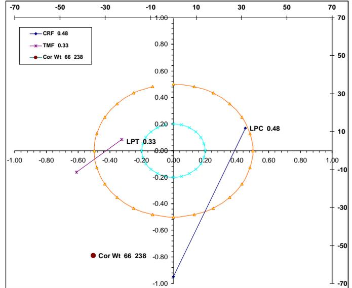
Figure 3. Predicted Vibration Levels for Initial Weight Vector
