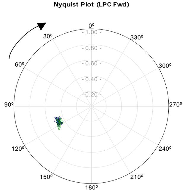
**Figure 6. Nyquist Plot Showing Magnitude and Phase Drift**
