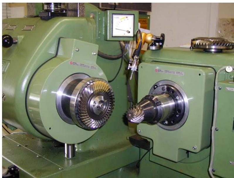
Figure 4 Microphone positioned above gearset mounted on input and output spindles.
