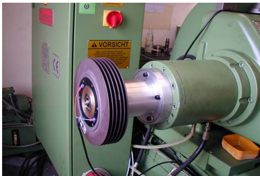
Figure 5 Magnetic particle brake assembly.
