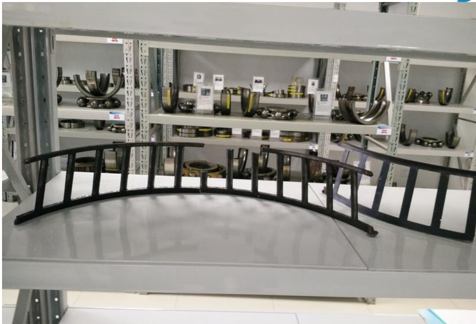
Bearing cage broken
