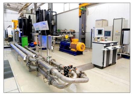
a PLC to control the test stand. It was necessary to offer a Profibus-DP interface to the PLC and in parallel a Ethernet interface to the signal conditioning system.
