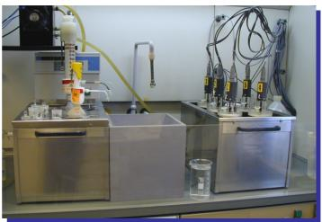
precise timed steps. The hydration heat, measured in calorimeters over periods of hours or days is a dimension for the quality. With the modules e.bloxx A5-1 temperatures get very precise recorded. The controller e.pac controlled the time flow, started the agitation motors in the 6 calorimeters, visualized and stored the measured values and makes these via Ethernet available to the server of the institute. The programming of the e.pac was realized with the graphical tool e.con.
