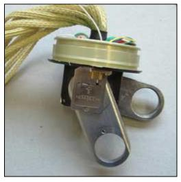
Sourced as an enquiry through our F312 shear pin design form web page, the customer required a small 22mm diameter shear pin loadcell to measure forces of up to 40kN. The loadcell would replace an existing pin in an ejector seat drogue parachute linkage. As the drogue parachute canister was launched with an explosive charge the loadcell would require protection to >1000 'g'.
